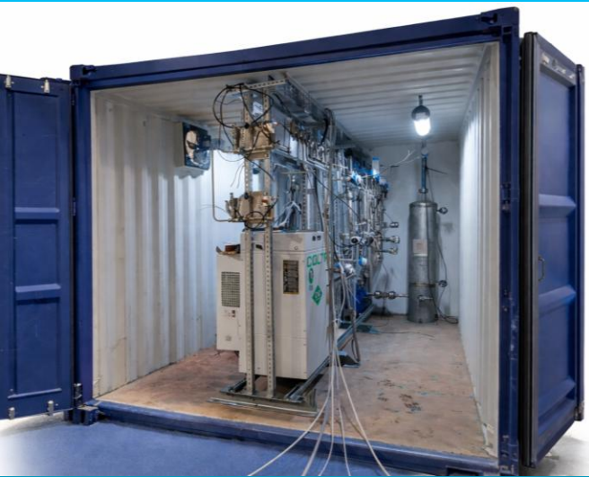
Containerized pilot plant for e-methane and e-methanol production
